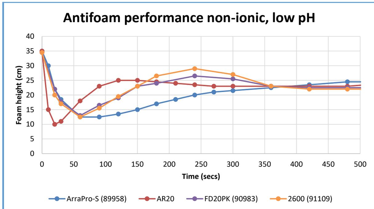
Figure 1: Antifoam performance of ArraPro-S in a non-ionic, low pH media compared to older products.
